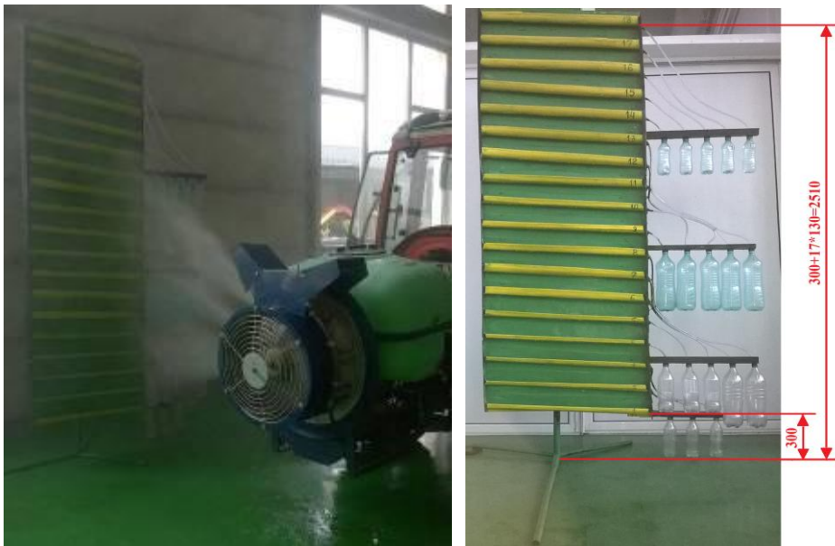
Fig. 1 Stand for determining the distribution uniformity of the dispersed pesticide fluid
